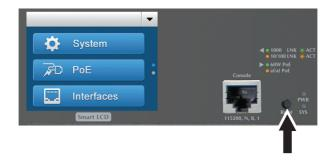
Figure 8-1: GS-5220 LCD Series Reset Button
