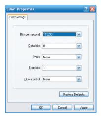
Figure 3-2: COM Port Configuration
